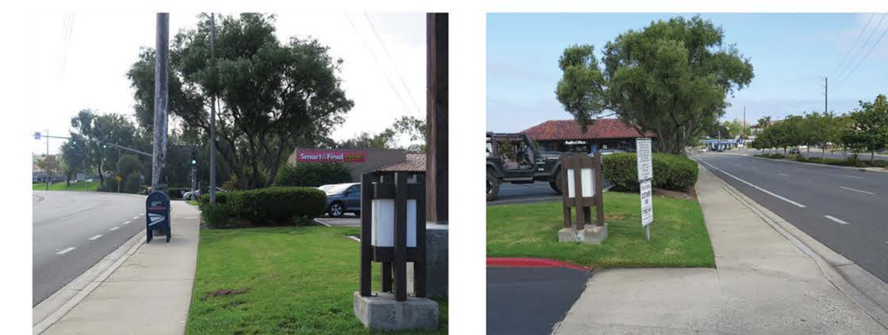
Sidewalks are attached to the curb with a generous landscape "buffer" between the sidewalk and the buildings.
