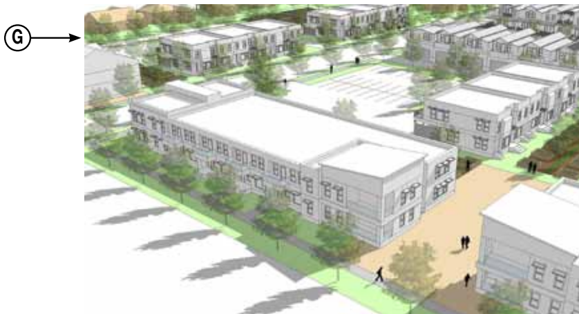
Locate a building to create a well-defined street frontage and minimize the visibility of parking areas.
