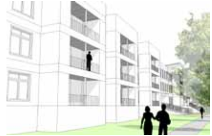
Provide vertical articulation in a larger building mass to establish a sense of scale.
