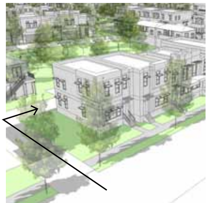
Provide auto access from an alley, rather than the street, when feasible.
