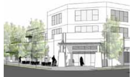
Use moldings, a change in material, or an offset in the wall plane to define the scale of lower floors in relation to the street.
