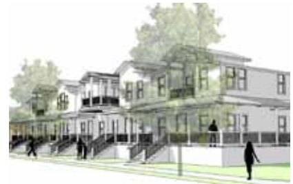
Organize modules to reflect traditional lots widths or facade dimensions that are seen in the area.
