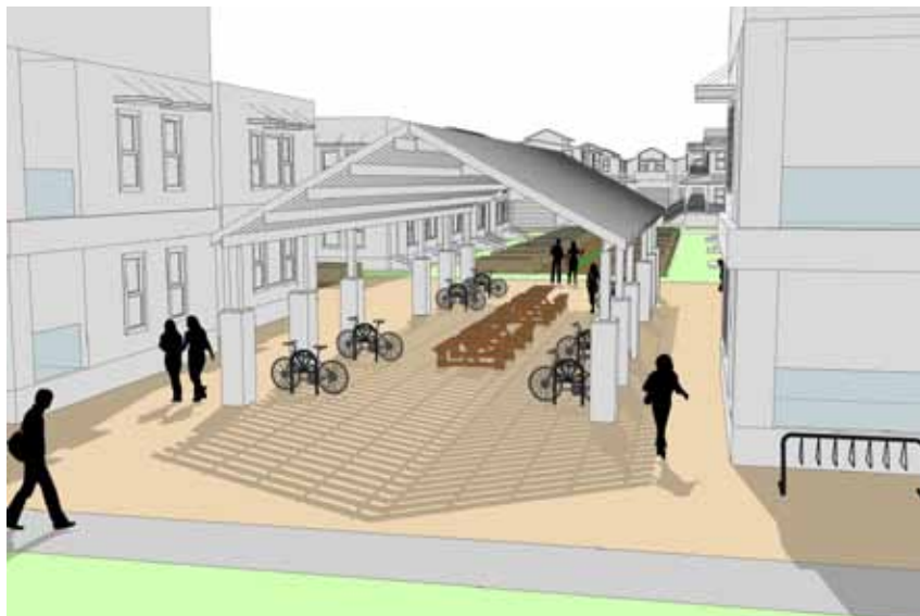
For a large residential project, incorporate both short-term (for guests and quick trips) and long-term (residents' permanent bike parking storage) bike parking.
