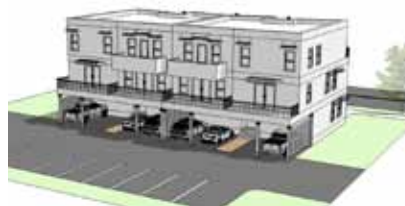
The three-story flat includes four tuck-under parking spaces per every six units. Extra on-site surface parking may be required.
