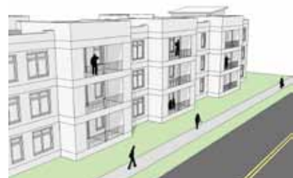
Locate features on the street facades that encourage interaction and thereby provide “eyes on the street.”
