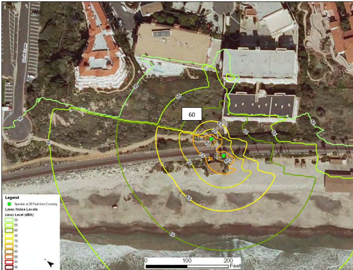
Figure 14—2. Typical Sound Distribution from AWS at a Crossing. Shown is the Corto Lane Crossing.
