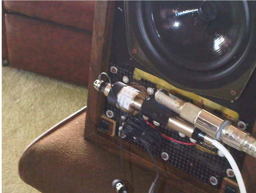
Photo 9—2. Earbud Inserted into Ear Simulator In Front of Excitation Source
