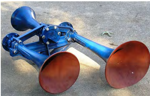
Photo 7—4. Leslie RS3L Three-Chime Train Horn
