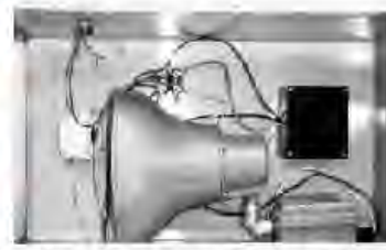
Figure 3. Automated Wayside Horn
