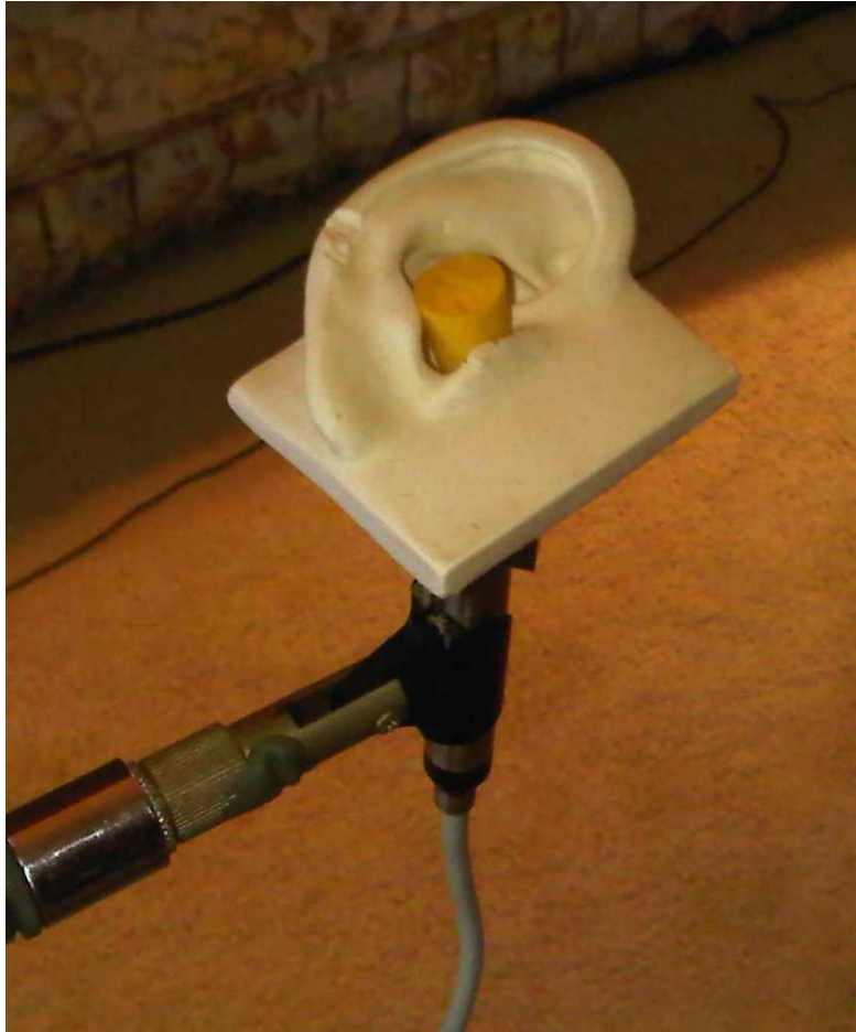
Photo 21—3. Close up of KEMAR Rubber Pinna Used for Testing the Loose Fit, Flat-faced Concha Type Earbuds. Shown with EAR© Insert Hearing Protector (earplug) Tested as a Control
