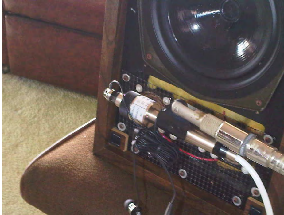
Photo 21—2. Earbud Inserted into Ear Simulator In Front of Excitation Source
