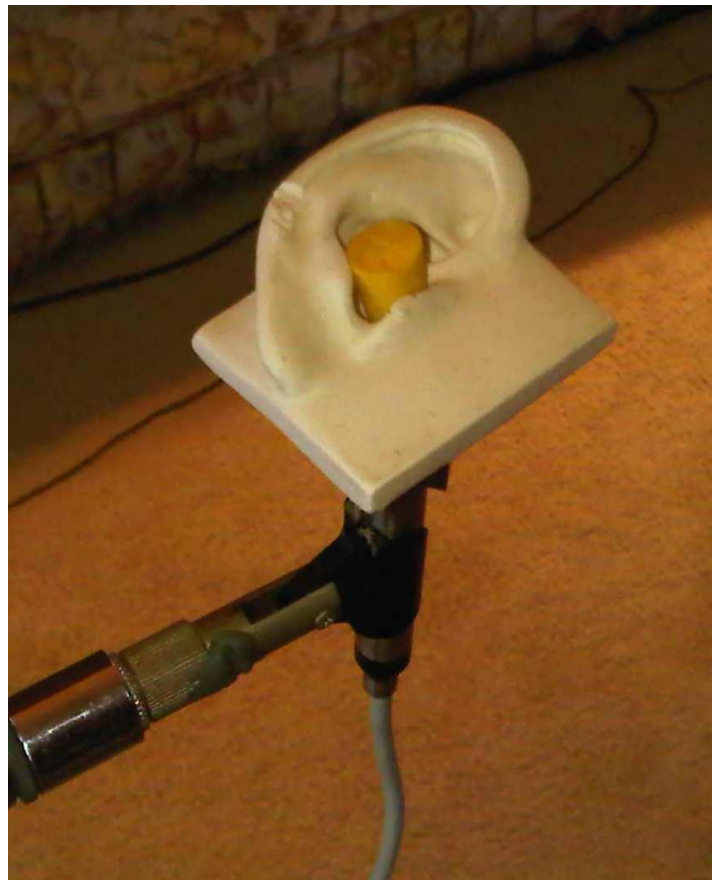
Photo 9—3. Close up of KEMAR Rubber Pinna Used for Testing the Loose Fit, Flat-faced Concha Type Earbuds. Shown with EAR® Insert Hearing Protector Tested as a Control
