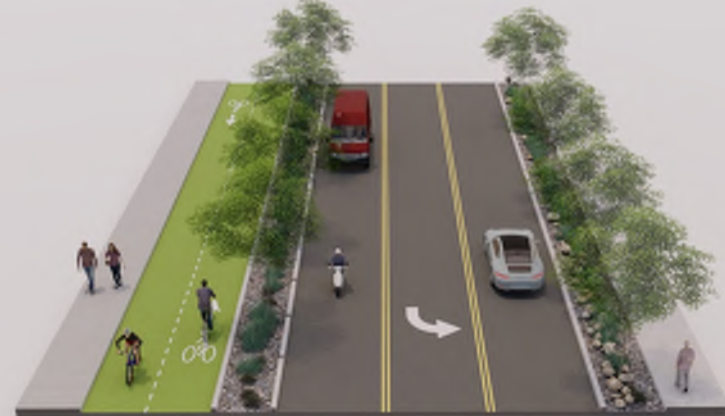
Class 4: Two-way Protected Bike Facility (Cycle Track)
