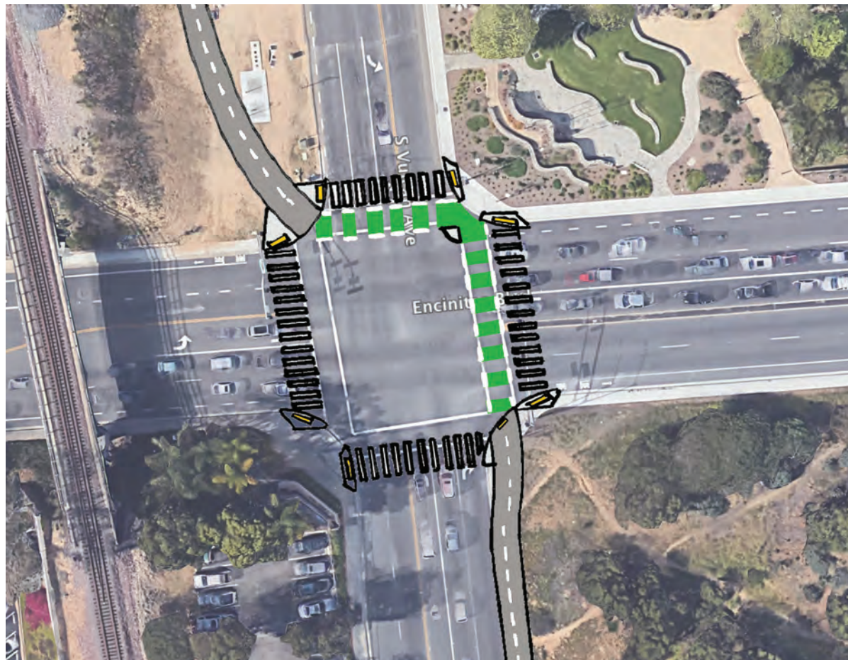
FIGURE 3-27: Protected Intersection Conceptual Design for Encinitas Boulevard at Vulcan Avenue
