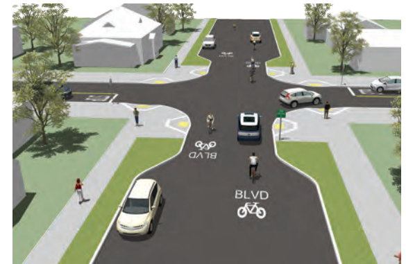
Class IIIB Bicycle Boulevard (Showing intersection vehicle diversion)
