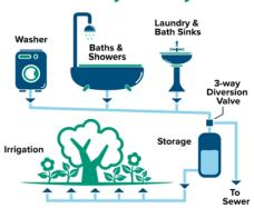
Typical graywater systems are onsite wastewater systems that use untreated graywater for subsurface landscape irrigation through the use of mulch basins, disposal trenches or subsurface drip irrigation fields.
