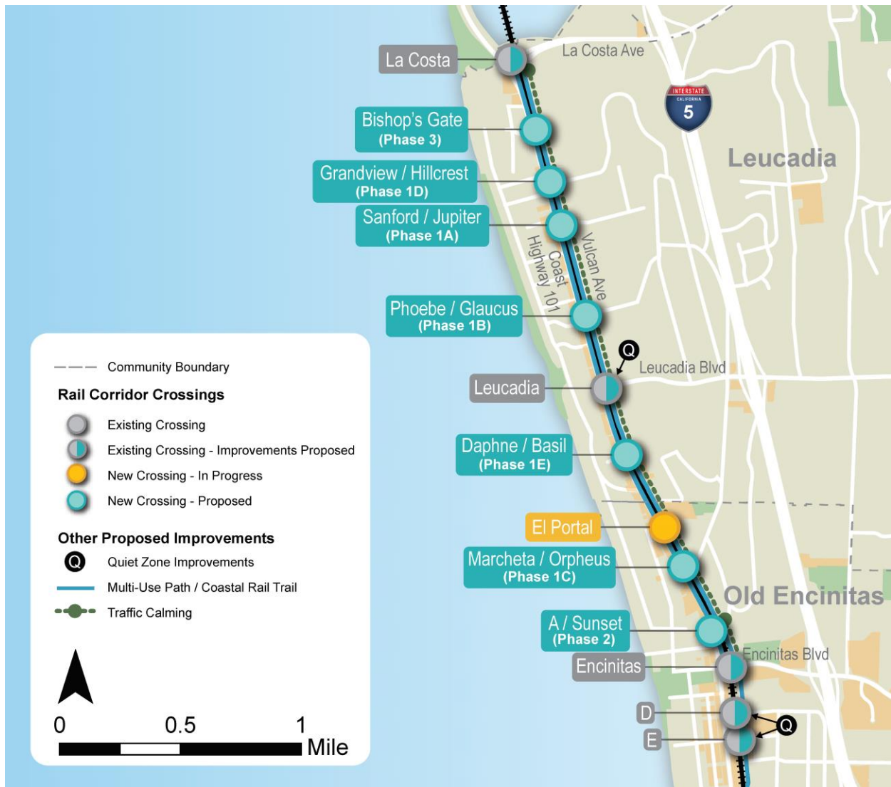
Figure 19: Proposed Improvements, North. Leucadia features a system of rail corridor crossings connected by the Coastal Rail Trail and a second multi-use path on opposite sides of the railroad tracks.
