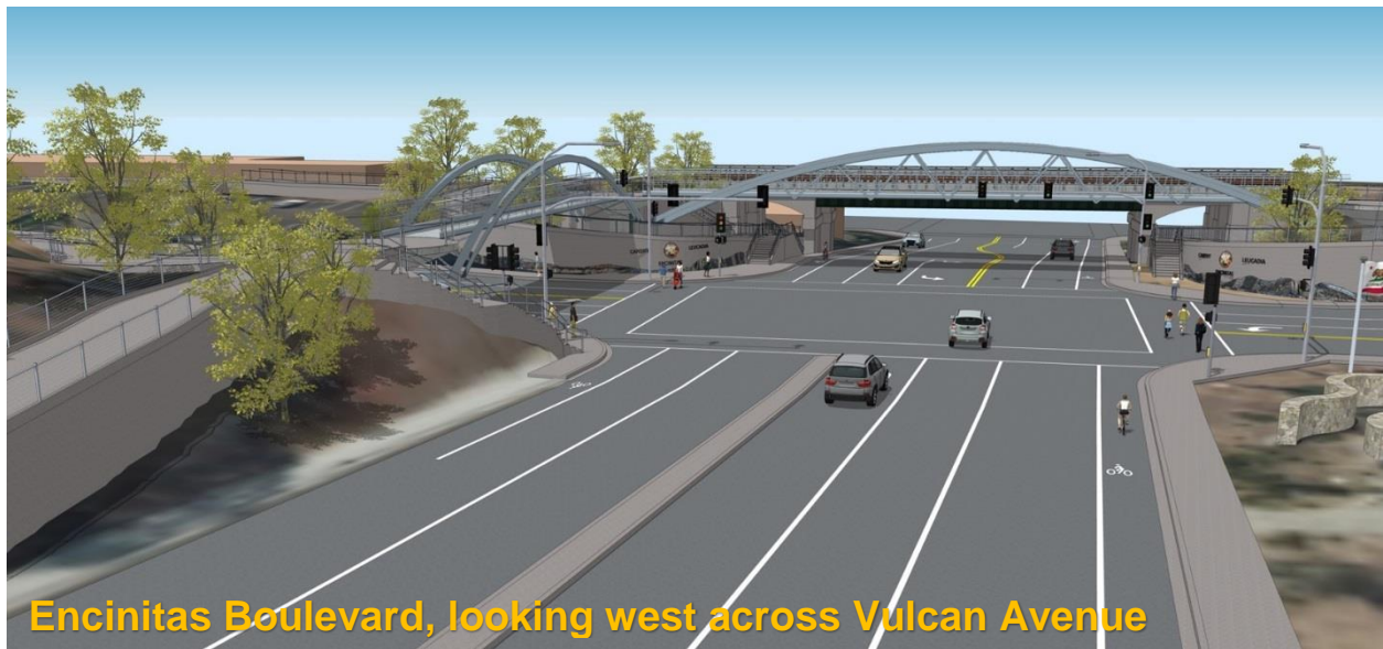
Figure 18: The proposed long-term improvement for the Vulcan Avenue multi-use path at the intersection of Encinitas Boulevard is a set of bridges separating cyclists and pedestrians from motorized traffic.
