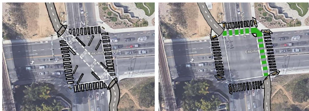
Figure 17: The proposed near-term improvement options for the Vulcan Avenue multi-use path at the intersection of Encinitas Boulevard include a diagonal “scramble” crossing (left) or a “Danish intersection” crossing (right).
