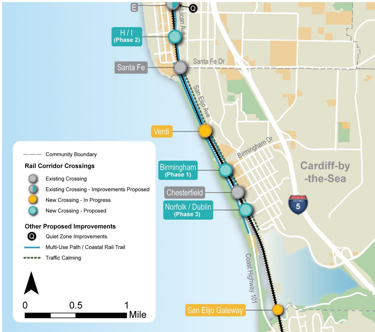
Figure 20: Proposed Improvements, South. Cardiff improvements include the Coastal Rail Trail east of the railroad tracks and a multi-use path along the coastal bluff west of Coast Highway 101.
