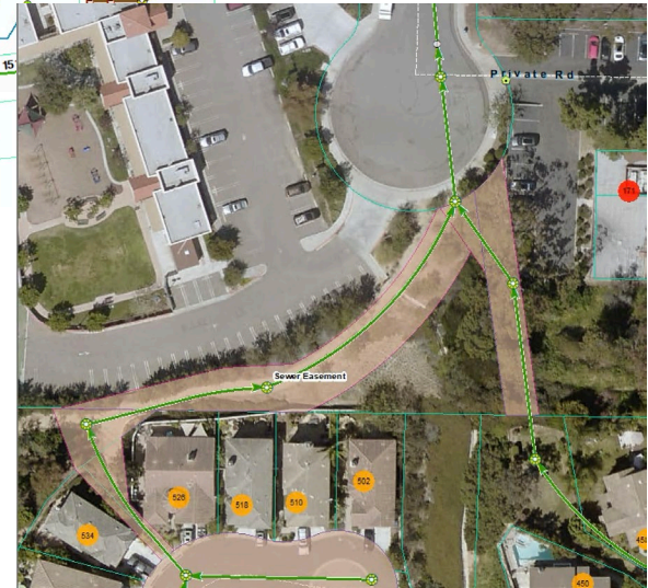
Sewer Pipe within Sewer Easement
