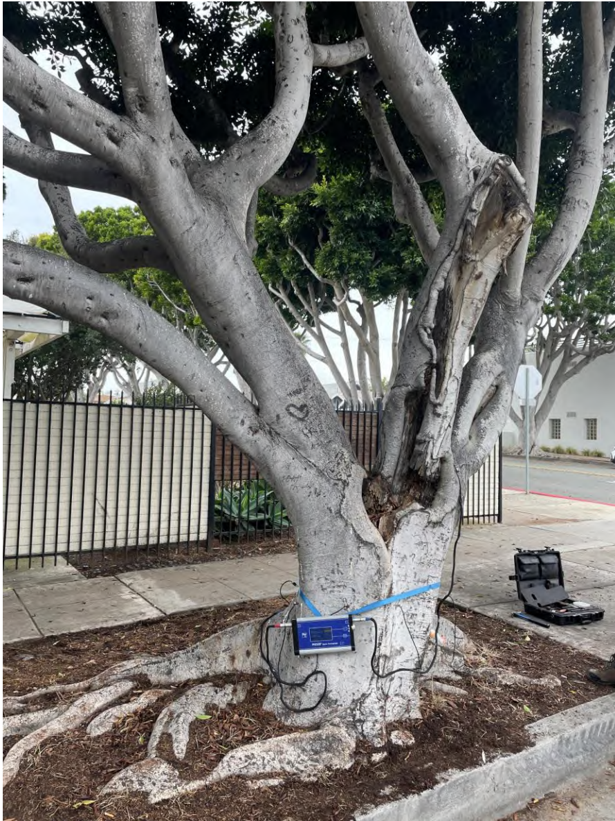
Detail photo of measuring points placed at 24 inches above soil grade and of heartwood decay in stem
