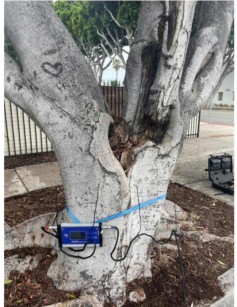
Detail photo of measuring points placed at 30 inches above soil grade and of heart wood decay in codominant stem union
