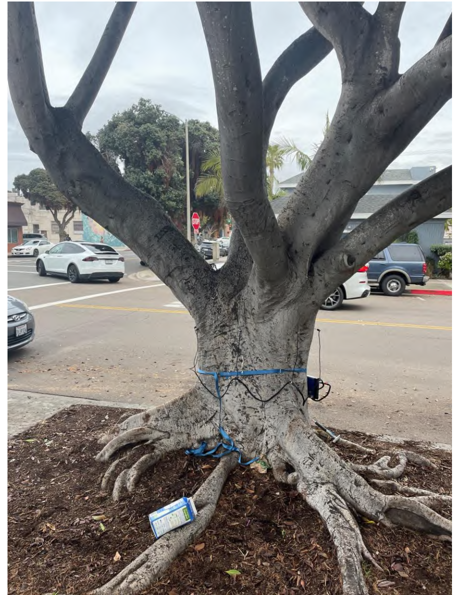
Trunk and sonic tomography unit facing northeast
